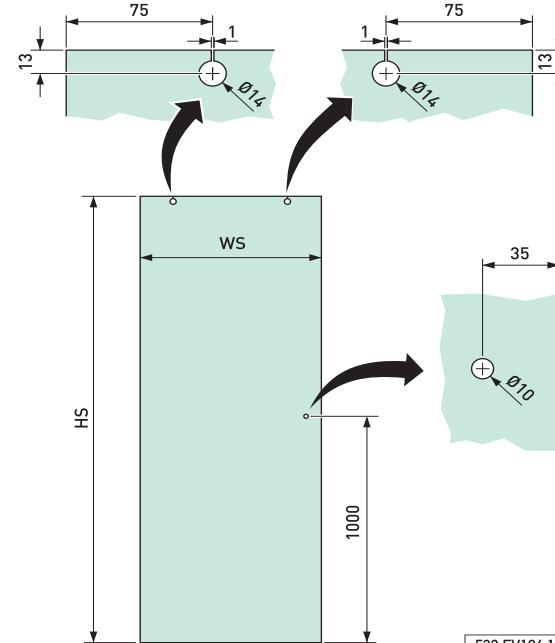
Only make the 10 mm glass drill hole if using the Aquant handle.
