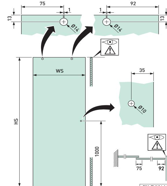
Only make the 10 mm glass drill hole if using the Aquant handle.
