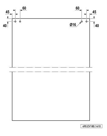
Drill holes 2<sup>nd</sup> sliding sash (with floating floor guide)
