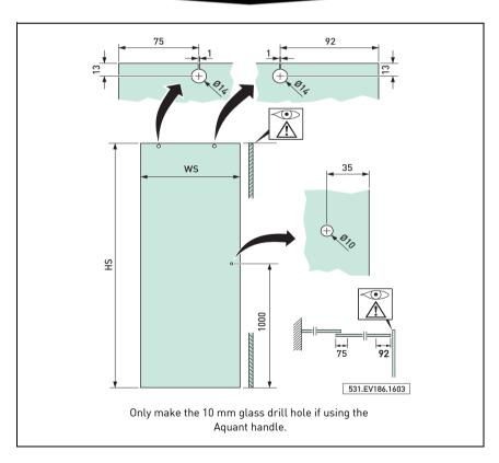
Aquant 40 - Glass drill holes for installation situations with glass panel bracket on one or two sides or with sliding splash panel
